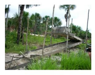
Figure 10-Wooden chute to separate gold
