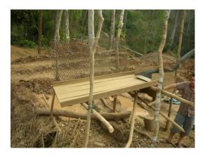
Figure 16- A wooden pellet covered with a screen to harass gold particles
